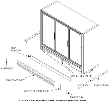
Figure 11A: Installing the bumper and kickplate
