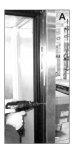
**A.** Back-out and retain the frame screws that secure the "J"-strip that covers the inside edge of the trim piece. If the door hinges on the side of the edge trim that needs replaced, it will be in the way of the frame screws, and will need to be removed first in order to access the screws.
