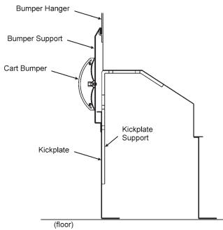
Figure 11B: Bumper and Kickplate Configuration
