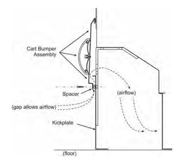
Figure 12: Bumper/Under-case air flow
