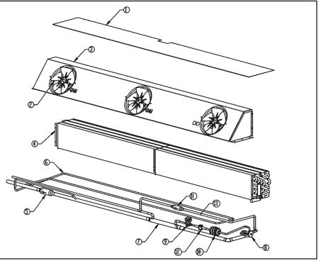
Figure 23: Coil Parts Breakdown, Hot Gas Defrost
