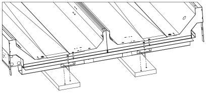
Figure 6: Removing wood planks
