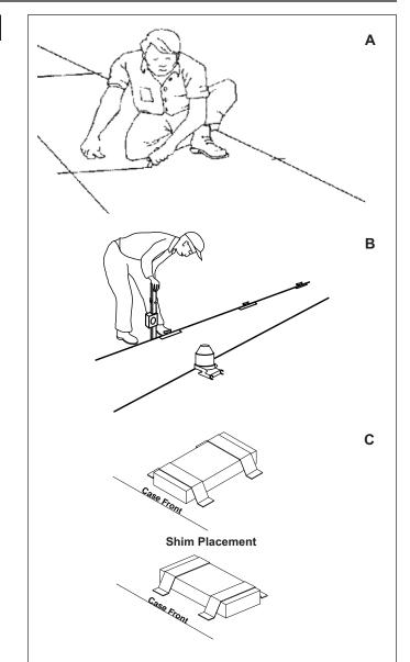
Figure 2: Leveling cases prior to joining
