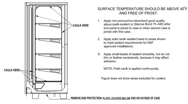
Figure 10: Required sealing for NSF approved installations
