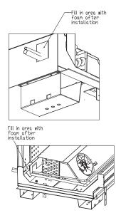
Figure 13: Penetration sealing
