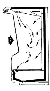
Figure 3 depicts what happens to the air flow in a case full of peg bars. The air falls through openings between packages and fails to maintain a protective "Air Skreen". When the bars are fully stocked, the effect is
