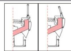
5-1/2" straight or 3-1/2" angled tempered thermopane glass front provide flexibility of front styling without reducing product visibility.
