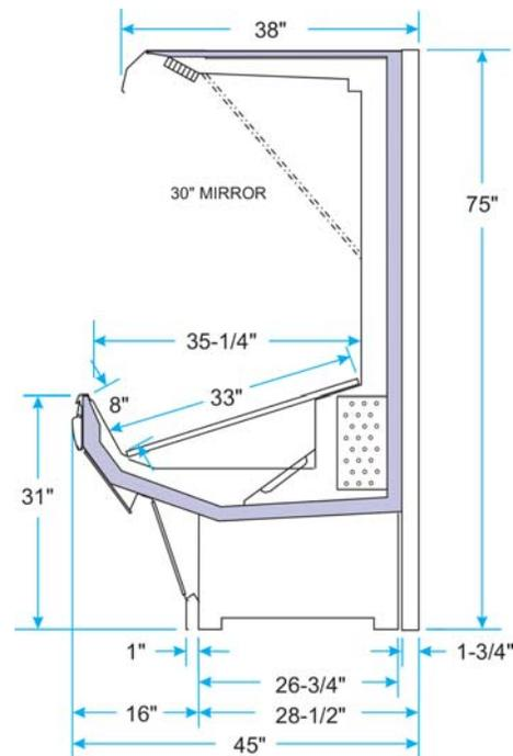
Allow a 3" SPACE between the back of this case and the store wall, other cases, or coolers to minimize possible condensation problems. FORCED VENTILATION may be necessary in some situations.
