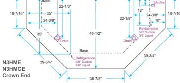
NOTE: There are four separate Suction & Liquid Refrigeration Line connection points in this case. All Refrigeration Lines can connect to either side of the adjoining case-to-case lineup. The access holes in the back of the N3HME or N3HMGE case line up with the access holes in the ends of the N3HM or N3HMG case.
