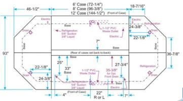
Island footprint shows back-to-back N3HM's or N3HMG's with two N3HME or N3HMGE crown ends
