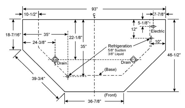
**NOTE:** There are four separate Suction & Liquid Refrigeration Line connection points in this case. All Refrigeration Lines can connect to either side of the adjoining case-to-case lineup. The access holes in the back of the N3MGE case line up with the access holes in the ends of the N3MG case.
