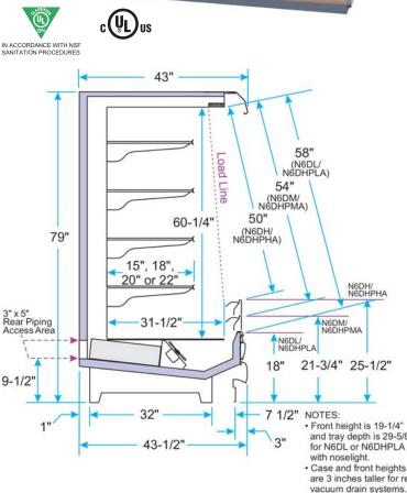
and tray depth is 29-5/8" for N6DL or N6DHPLA · Case and front heights are 3 inches taller for rear vacuum drain systems.
