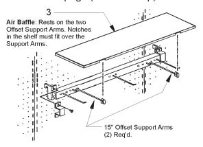
3. Non-load bearing air baffle should run the same width as the peg bar. Air baffle rests on the two offset support arms. The notches in the air baffle must fit over the support arms. NOTE: The air baffle should be solid in design and positioned 1" in front of the rear duct and 5.5" back from the rear edge of the card moulding.
