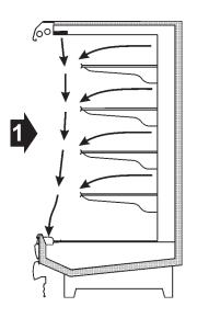
Figure 3 depicts what happens to the air flow in a case full of peg bars. The air falls through openings between packages and fails to main-
