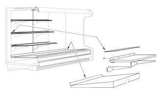
All egg shelves come galvanized or stainless steel. The upper egg shelves are 15" x 48" and come with 82 degree fixed white brackets. The brackets are available in one position only. The upper egg shelves assemblies include a rear air close-off.
