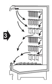
tain a protective barrier. When the bars are fully stocked, the effect is minimized, but product temperatures will not be as good as they could be. Sweating may be noticed on the top duct panel above the bars. The coil will also frost faster, requiring more frequent defrosts.
