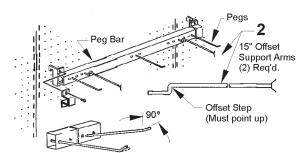
Pegs: After marking the desired locations for the Pegs on the Peg Bar, insert the Pegs by holding them at 90 °, and insert into the holes so Peg points are up. Pull out Peg to seat properly on the Peg Bar.
