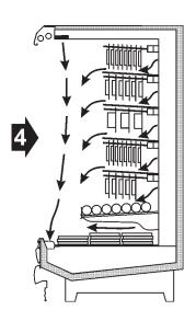
Figure 4 shows the proper air flow for cases with peg bars. The addition of a baffle above each row of peg bars, except the top row and a bottom shelf, maintains proper air flows and temperatures in the case. Nonload bearing air baffles should run the same width as the peg bars.
