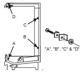
All N7DNHPL and NHDHP models have four pull-ups at each end of the case. Pull-ups A, B, C and D are located as shown and should be installed and tightened starting with A and finishing with D.
