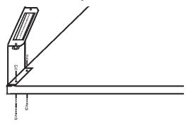
4. Mount the bracket to the bottom tray with two screws, washers and capnuts.
