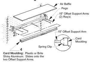
4. Card moulding is offset 2" in front and 3/4" above the pegs.
