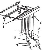
If the wiring harness has not been factory installed, remove insulation from top of center riser and lay wire harnesses (1) on top of the center partition (2). The 8' harness has three female plugs and one male plug. The 12' harness has four female plugs and one male plug. There is one harness for shelf anti-sweat heaters
