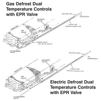
connected directly to the compressor suction that allows for low temperature operation. When the solenoid is closed, the evaporator must operate through the EPR valve which has been preset to the desired medium temperature.
