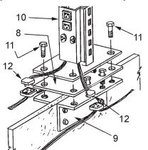
Install and align the center upright (10) to base plate (8) and angle brackets (9) with four bolts (11). (The four corner bolts are used for adjusting the center uprights.) The center uprights may face in either direction. Connect upright wire plugs (12) to harness. Route wires and harness around the uprights in the insulation.
