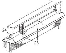
10. Install top riser caps (23) on top of the center partition. Drill pilot holes in the top center of the two riser caps and secure with screws (24).
