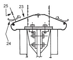
Position card moulding (25) as shown and drill 1/8" pilot holes in riser caps (23).
