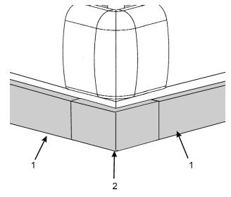
After kickplates (1) have been installed, position kickplate corner trim (2) over both ends of the kickplates (1) and secure with screws.
