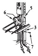
Position the RH end post (5) in the RH superstructure hole in the center riser (3). Install the two plugs (6) and push them into the insulation. Push down the RH end post (5) until it seats into the center riser (3) and secure with four bolts (7).
