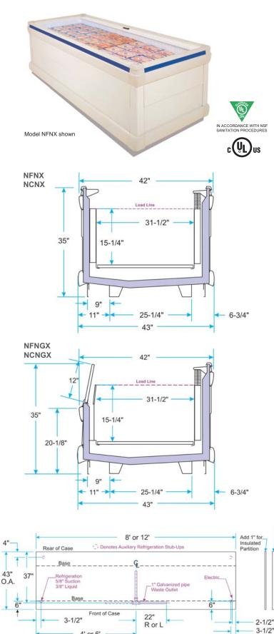
NFNX, NCNX, NFNGX, and NCNGX island merchandisers provide a narrow 43" depth where floor space is limited. The NFNX and NFNGX can display frozen food or medium temperature products, while the NCNX and NCNGX are designed for either frozen foods or ice cream products.
