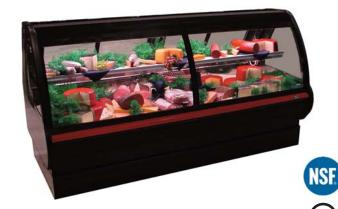
NFD service merchandisers provide forced air, lower-coil cooling that maximizes product integrity. A single sealed triple-pane front glass offers seamless front viewing while increasing the case's insulating factor, providing an energy-efficient alternative to lift glass versions.
