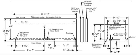
**STUB-UP NOTE:** One floor drain can serve up to two cases per drain. One electrical stub-up can serve a number of cases depending on the circuits required – utilizing the continuous wire raceway(s) on the front of the cases. One refrigeration stub-up can serve several or all cases on a line-up with case-to-case piping. Maximum 1 5/8" for case-to-case piping.
