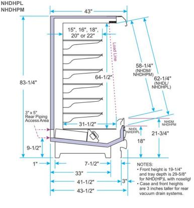
ALLOW 3" SPACE between the back of this case and the store wall, other cases or coolers to minimize possible condensation problems. FORCED VENTILATION may be necessary in some situations,
