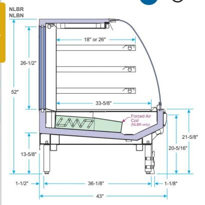
NLBR bakery service merchandisers provide forced air, lower-coil cooling that maximizes product integrity. The NLBN is a non-refrigerated version. The front curved glass is designed to maximize product viewing, while the glass lift system allows easy front access for stocking and merchandising of baked goods.
