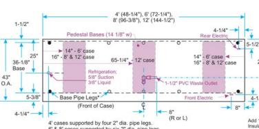
6' & 8' cases supported by six 2" dia. pipe legs 12' cases supported by eight 2" dia. pipe legs
