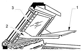
To install mezzanine shelving, position and insert the mezzanine shelf (1) and captive shelf brackets (2) into slots in the uprights (3).
