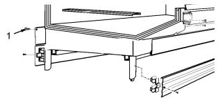
Position rear rail cover (1) over rear raceway opening and secure with screws in every hole.
