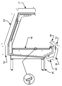
The joint trim and mounting hardware are shipped loose. Trim includes top joint trim (1), rear upper joint trim (2), rear lower joint trim (3), front kickplate joint trim (4), front lower cladding joint trim (5) and front upper cladding joint trim (6), color band backer (7), hand rail joint trim (8) and horizontal joint trim (9).
