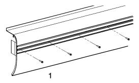
1. Install bumper retaining track on cladding with screws, if required, using same alignment as old bumper track.
