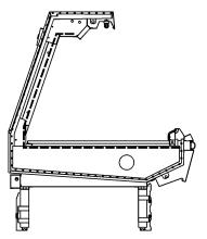
Apply two heavy beads of caulking compound from the Filler Kit to the end of case at dotted (. . .) and dashed (- - -) lines. Proper caulking provides good case refrigeration and sanitation.
