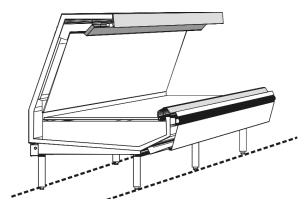
1. Snap chalk lines where the front and rear of the case legs are to be located for the entire line-up.
