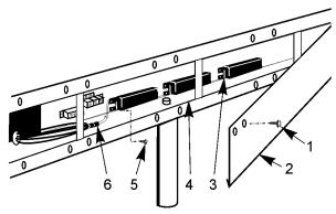
1. Remove screws (1) and rear rail cover (2) from rear of case.
