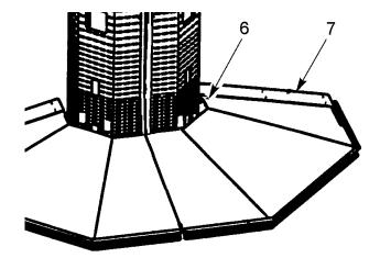
Loosen set screws (6) in top of end Tstrips (7). Position end T-strips to connect and cover space between shelves. Tighten set screws (6).
