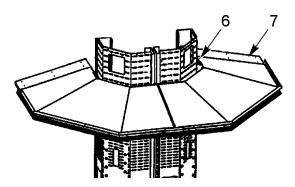
Loosen set screws (6) in top of end Tstrips (7). Position end T-strips to connect and cover space between shelves. Tighten set screws (6).
