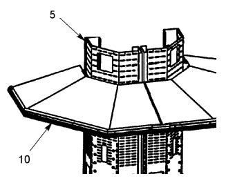
Install upper shelf & bracket assemblies (10) in outside slots (5) in rear duct.
