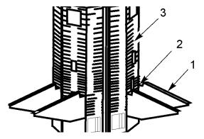
Position center shelf brackets (1) in desired center slots (2) in rear duct (3).
