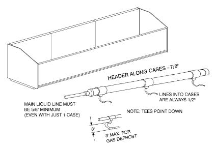
Liquid lines to the cases should be branched off the bottom of the header. This ensures a full column of liquid to the expansion valve. A branch line from the header to an individual case should not be over 3' long and must have 3" expansion loop incorporated.
