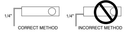
If an evaporative condenser is used, the sensor should be mounted in the evaporative condenser sump. The sensor should be halfway submerged in the sump water with the pilot line connection pointing downward. *(Refer to page 24-28.)*
