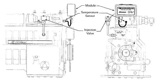
FIGURE 1 DEMAND COOLING SYSTEM COMPONENTS (REPRINTED FROM COPELAND ENGINEERING BULLETIN AE-1287)
