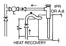
As shown, the outlet pressure from the heat recover coil is exerted on the underside of the bellows and the top of the seat disc at the same time. Since the effective area of the bellows and the disc are the same, the two pressures cancel out. The force of the incoming pressure alone will work against the spring pressure to operate the valve.
