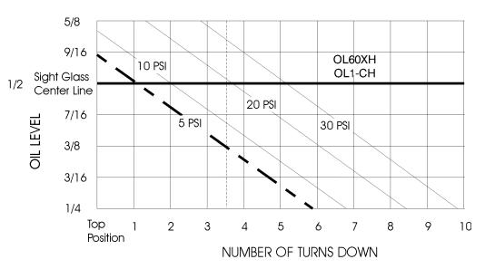
NOTE The oil level control is factory set at 3-1/2 turns clockwise from the top stop.
