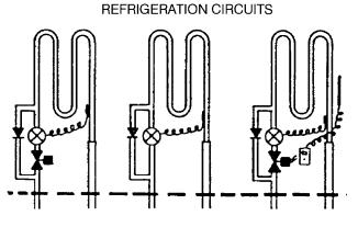
A Refrigeration Branch Circuit is a lineup or group of cases and/or coolers connected to a common liquid line solenoid and common suction line. The suction line may or may not be equipped with an EPR valve.
