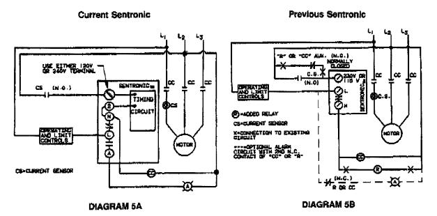
Both Diagrams 5A and 5B use a current relay (C.S.). When the current relay is not energized by motor current, its Normally Open (N.O.) contact opens the circuit that powers the Sentronic to avoid a nuisance trip.
