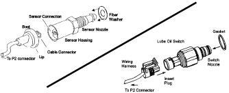
Figure 3: Sensor / Switch Installation
