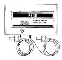
The P45 control measures the net oil pressure available to circulate oil through the lubrication system. (Net oil pressure is the difference between the oil gauge pressure and the refrigerant pressure in the crankcase.)
