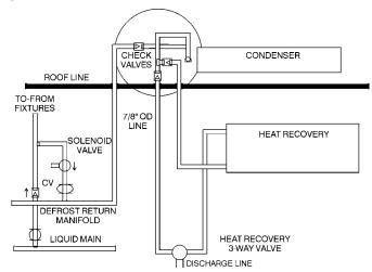
One check valve is mounted in the liquid line leaving the main liquid supply manifold. Its purpose is to allow liquid flow during refrigeration and block liquid flow to the main liquid supply manifold during a gas defrost.
