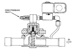
This normally open valve is operated from the multi-circuit time clock or computer controller. During the refrigeration cycle the valve is de-energized and remains open. The valve makes use of the system's low pressure to hold itself open by porting the top of the piston to suction manifold. When defrost is initiated, the solenoid valve is energized, directing system high pressure to the top of the piston, closing the valve.
