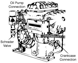
If the net oil pressure drops below the "heater on or cut-in" value during the running cycle, the time delay is energized. If the net oil pressure does not return to the "heater off or cut-out" value within the time delay period, the compressor will be shut down.
