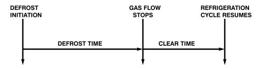
When the termination temperature is reached (70°-75°F), the hot gas solenoid will close. If the coil cools and the termination time has not elapsed, then the hot gas flow will resume. This will continue until the allotted failsafe time on the time clock or computer controller has been reached.
