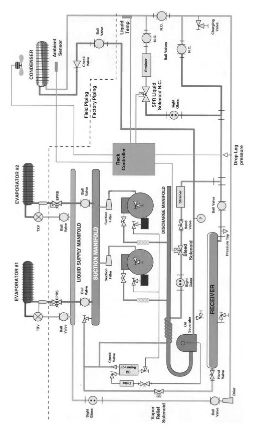
Enviroguard III Piping Diagram for Electric or Time Off Defrost Winter Operation
